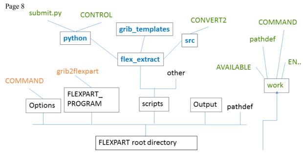
Fig. 1: FLEXPART directory structure (black) with directories in rectangles, files as text. flex\_extract software should reside in scripts directory. In order to create input files on height levels (.fp files) flex\_extract will need to have access to COMMAND file and grib2flexpart executable (red). Flex\_extract software will create directory work and place all output files there. Usually the work directory will reside on a separate large file system.
